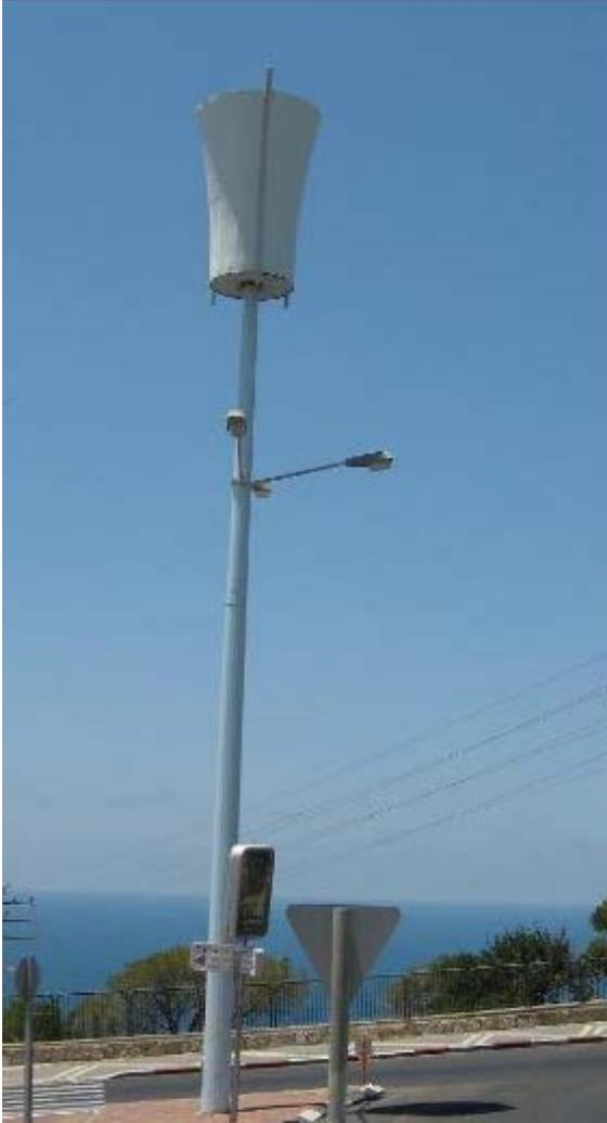
**Exhibit 8.** The antenna is wider than, and out-of-scale to the pole. This design is prohibited.
